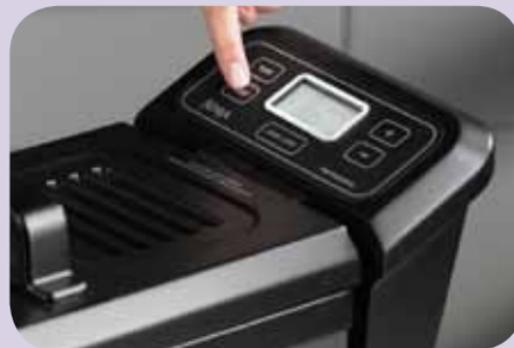
2. Press the TEMP button to enter the desired temperature
